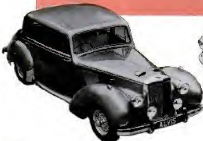
ALVIS Grey Lady, left, is a 100-mile-per-hour sedan with a high-compression, overhead-valve "square" engine and a seven-bearing crankshaft
